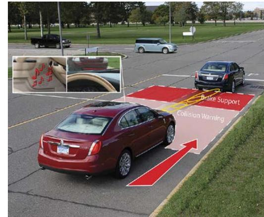
By Ford Motor Company from USA - Collision Warning with Brake Support, CC BY 2.0, <https://commons.wikimedia.org/w/index.php?curid=5069537>
